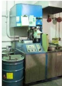
Through our solvent recovery system (the still), we reclaim and reuse waste acetone used by the finish department. The hazardous waste from the still is turned into a cleaning solvent that is sold to metal companies for cleaning products, greatly reducing the solvent waste shipped off site.
